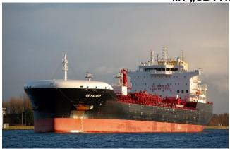
C/O-Tanker Ship Type: Deadweight: 37,874 tdw Built 2020 Phenolic Epoxy Coating Ship Class: DNV Length over all: 183 m
