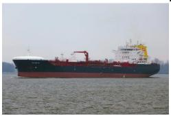
Ship Type: C/O-Tanker 37,874 tdw Deadweight: Built 2020 Phenolic Epoxy Coating Ship Class: DNV Length over all: 183 m Breadth: 32 m Draft: 10.5 m
