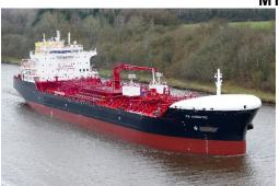
Ship Type: Deadweight: Built Coating Ship Class: Length over all: Breadth: Draft: C/O-Tanker 37,856 tdw 2019 Phenolic Epoxy DNV 183 m 32 m 10.5 m
